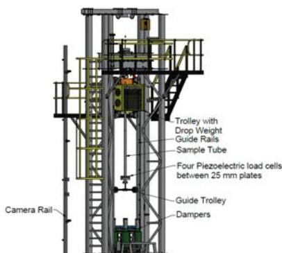
Figure 1 Schematic of Dynamic Impact Tester (DIT)
